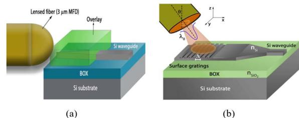
Fig. 2. Edge-coupling (a) versus Grating-coupling (b) photonics test setups for final product and wafer-level tests respectively [2].
