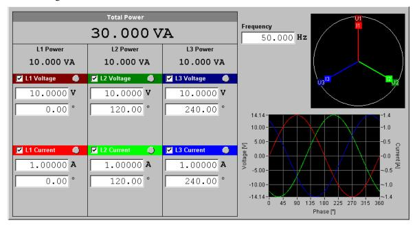
There are displayed channels of the calibrator in the left side - L1, L2, L3. Power is displayed independent for each channel and also as Total power. Each channel contains parameters of voltage and current outputs:
