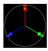
In the upper right corner is displayed vector diagram. There are displayed or current (I1, I2, I3) and voltage (U1, U2, U3) outputs. North pointing vector (position on the twelve o'clock) shows angle 0°. South pointing vector (position on the six o'clock) shows angle 180°. The picture shows outputs I1, U1 (angle 0°), outputs I2, U2 (angle 120°) and outputs I3, U3 (angle 240°).
