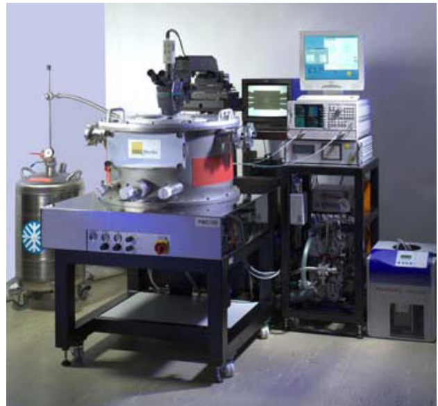
Fig. 1. The PMC200 cryogenic measurement system used for experiments.
